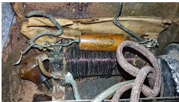
"Item #11: An internal view showing an induction coil and a capacitor within the object.
