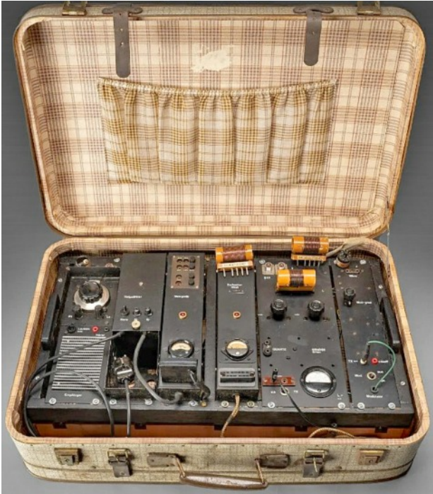
Item #4/1: This replica, roughly inspired by a Type 3 Mk.I (B 1), was well-crafted but lacked originality in almost any detail. The only apparent genuine items were the transmitter plug-in coils.
