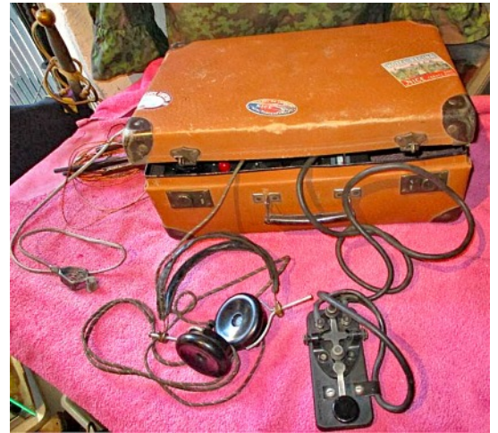
Item #7/1: Suitcase with headphones, Morse key and accumulator cable (right).
